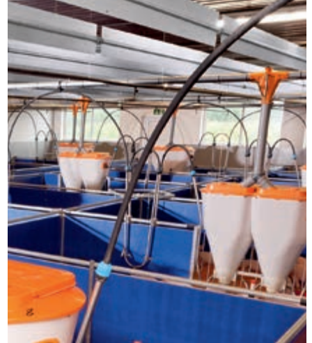
Twin pipe – less dust on pipes
